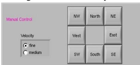
In the manual sector there are all control components required to control the motor. The velocity can be chosen by a radio button "Velocity". Eight available buttons correspond to 8 directions the telescope can move. Each button is a toggle. Pressing the "Guide-off"-button also stops moving the telescope.
